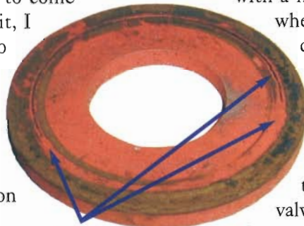
Note uneven grooves or wear patterns.
