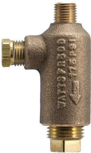
◀ Watts Series FR 500 Thermostatic Freeze Relief Kits are designed to keep water from freezing in the backflow preventer, while avoiding discharges based on the air temperature dropping below freezing. Series FR 500 thermostatically measures the water temperature and opens at 35°F (1.6°C) and closes at 40°F (4.4°C). Maximum Working Pressure: 175psi (12.06 bar).
